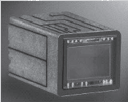
Figure 1 – micro camera (Courtesy of 3D PLUS)
